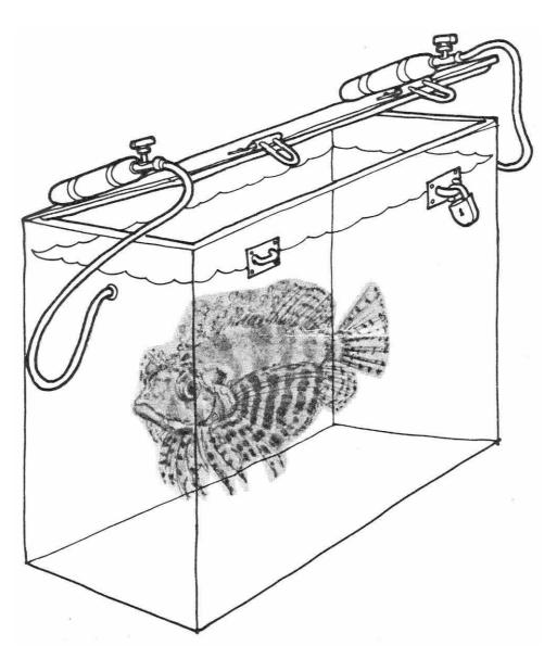
3.1 The container should be constructed of suitable gauge, rustproof metal and should be completely watertight. In certain circumstances, glassfibre containers would be more satisfactory.
