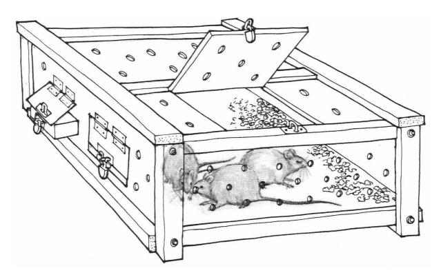
3.1 The container should be constructed of mesh-lined wood, or material of similar strength, and should be strong enough to house the animals, and to withstand the handling involved during transport.
