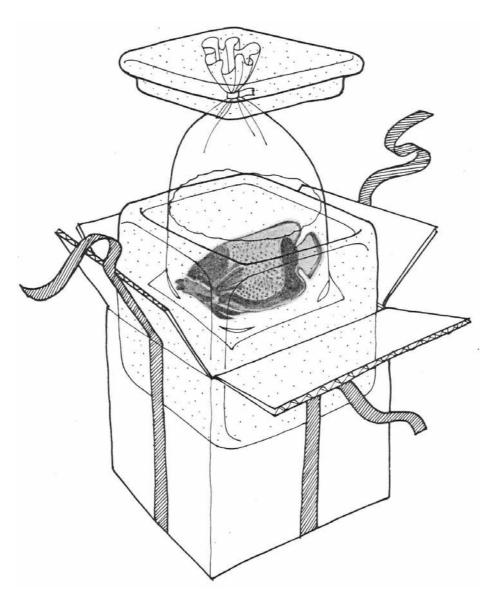
3.1 The container should be constructed of suitable, strong, high-density, expanded polystyrene, or material with similar strength and insulating properties.
